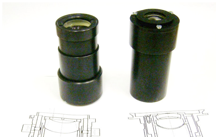
Figure 57 The finished optical assemblies for COLORES in the Turnov optical workshop. (left: camera, right: collimator).
